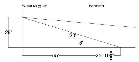
Note the characterization that a 20' high sound curtain barrier would offer 20-30 dBA of transmission loss compared to 10-20 dBA of transmission loss for a plywood barrier is incorrect and a mischaracterization of the barrier attenuation that can be obtained from a barrier with a direct line of sight between the source and a receiver.
