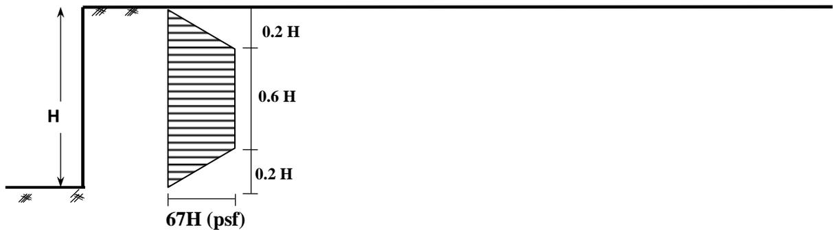
**Trapezoidal Distribution of Earth pressure Plus Hydrostatic Pressure**
