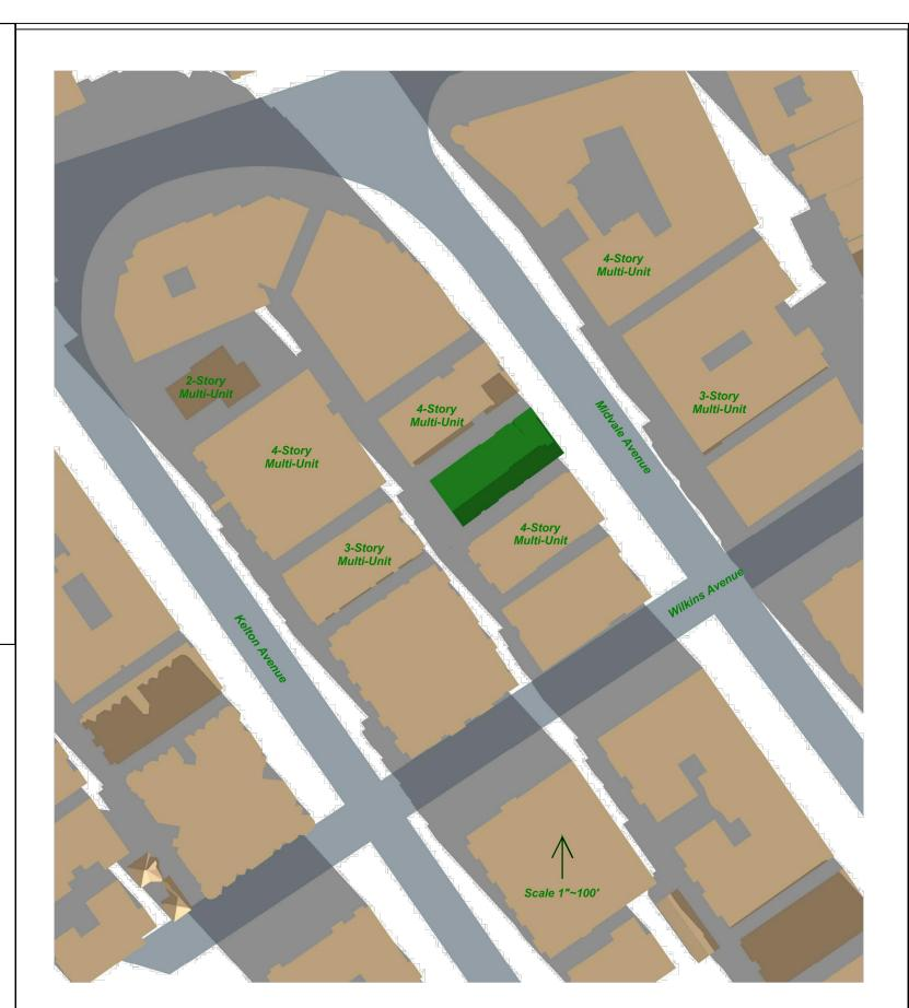
Winter Solstice Shading Diagram 9 a.m.
