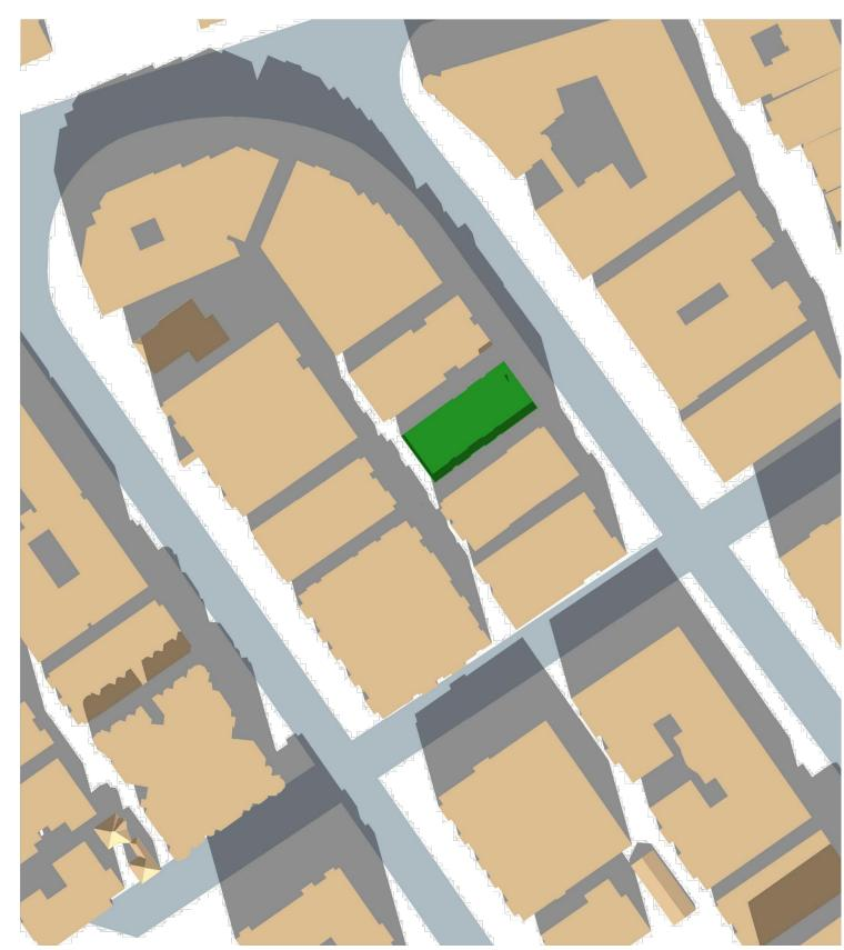
Winter Solstice Shading Diagram 11 a.m.
