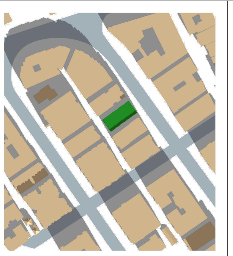
Winter Solstice Shading Diagram 10 a.m.
