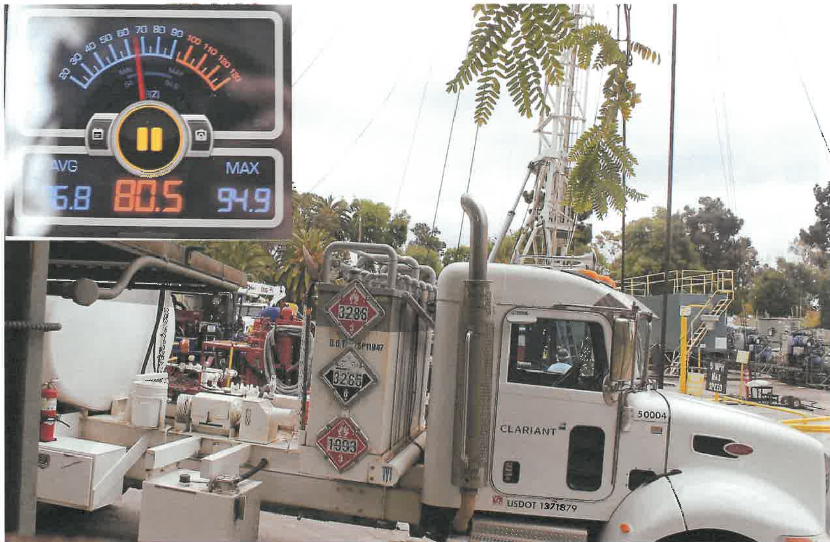
Figure 20 - A Clariant Acid Tanker parks next to the west wall. The workover rig works to pound a metal pipe into a well. A crane loads pipes onto a flatbed in the background. Peak decibels were 94+ with each pounding.
