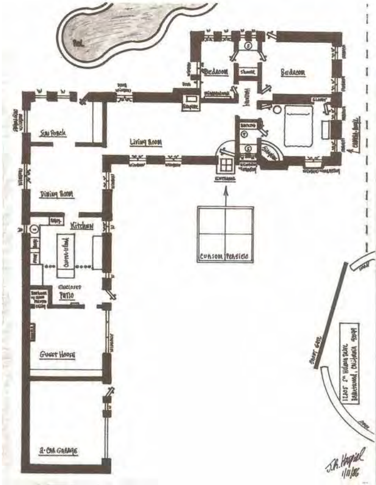
A contemporary floor plan depicting the organization of the main residence, garage, and guest house. The dotted line denotes the original boundary between the kitchen and the walled courtyard. Courtesy of CursumPerficio.net.
