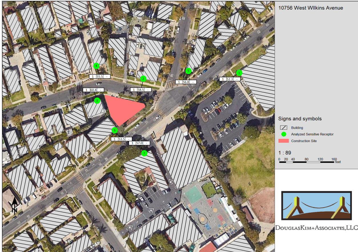
Figure 2 Construction Noise Levels at Sensitive Receptors
