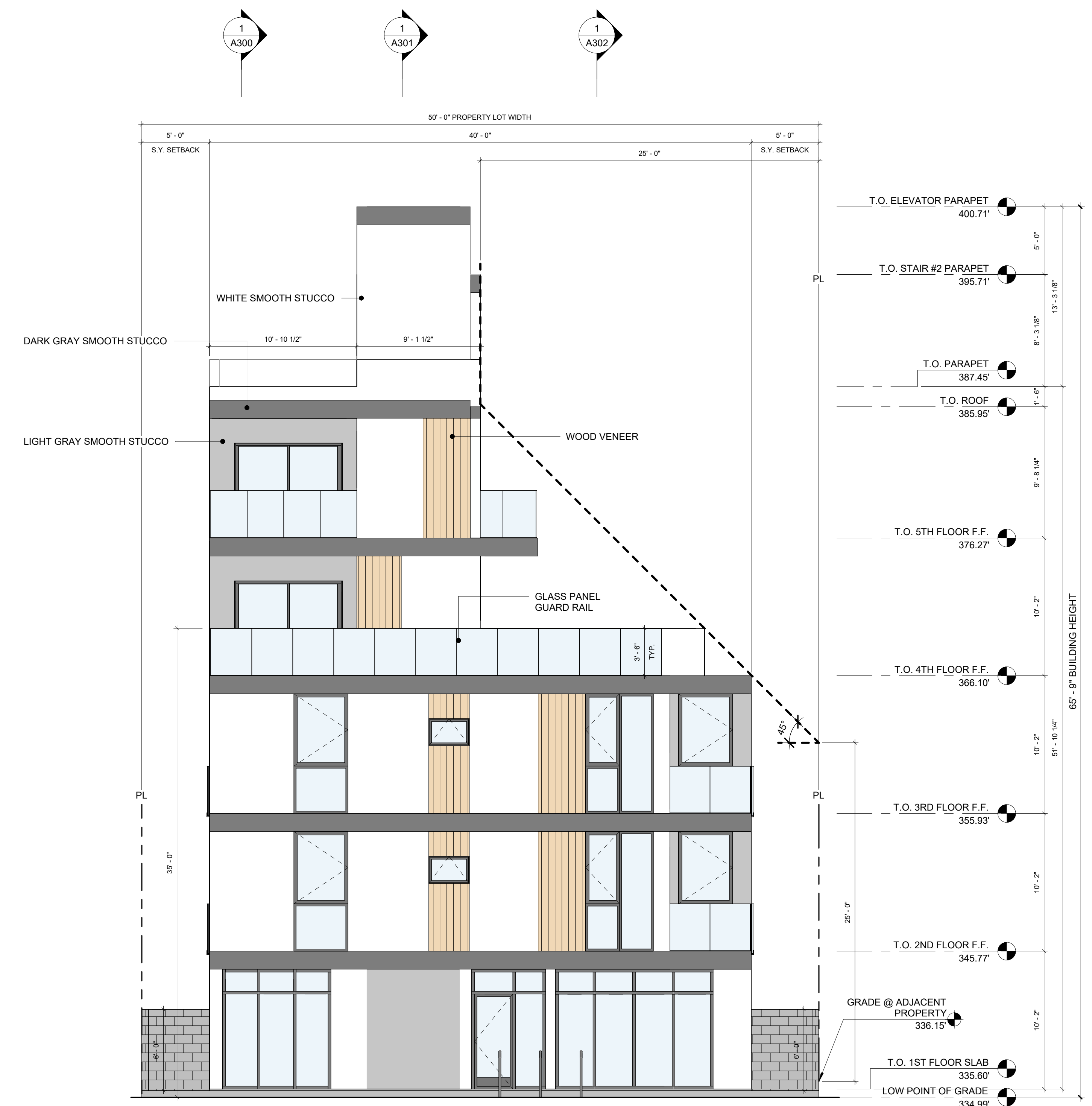
3 WEST EXTERIOR ELEVATION - TRANSPARENCY DIAGRAM 3/16" = 1'-0"
