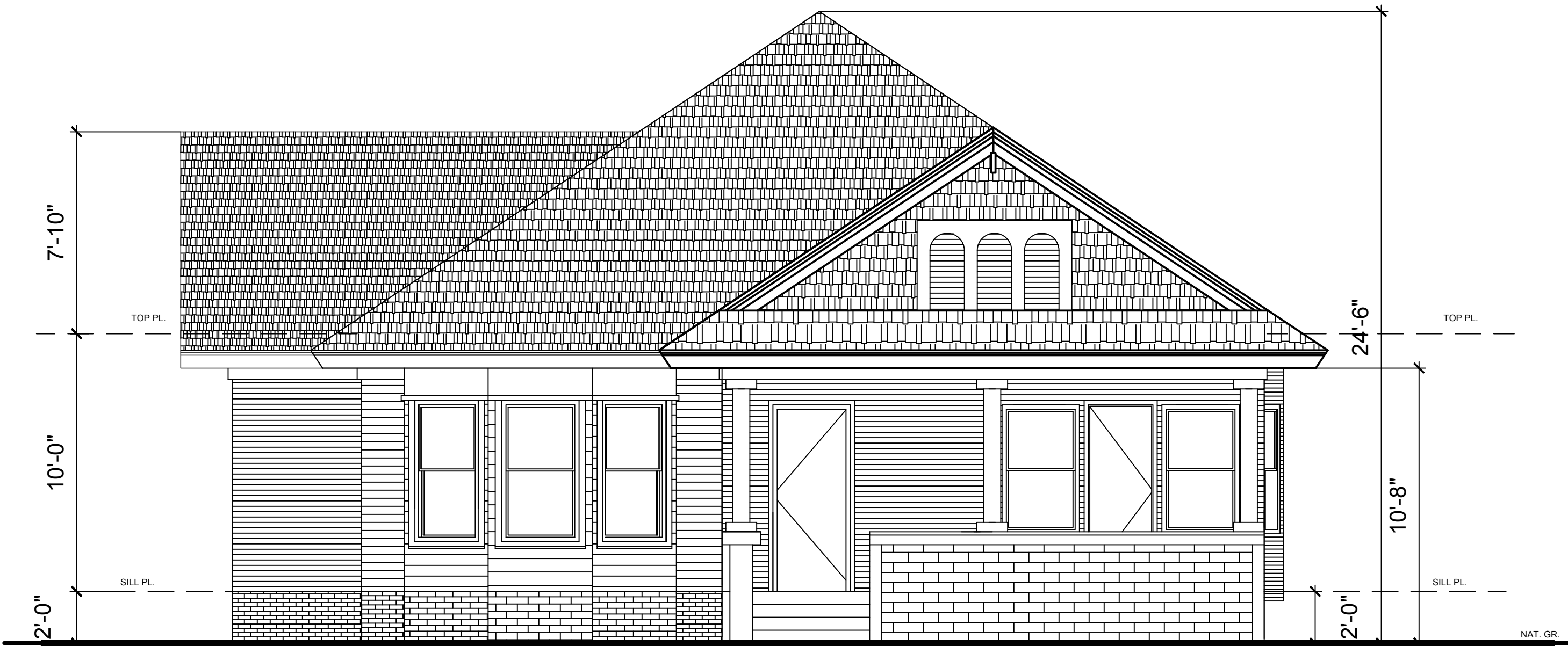
WEST ELEVATION VIEW sc: 1/4"= 1'-0"
